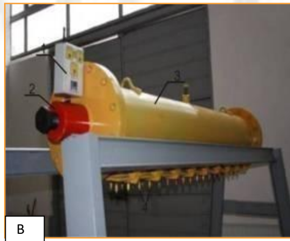
A - Water mist generator for horizontal dispersal; B - Water mist generator for vertical dispersal 1 - absorber control block, 2 - high pressure camera, 3 - water container, 4 - nozzles
