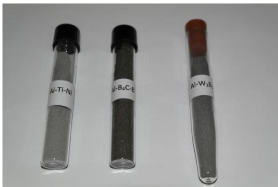
Powder mixture prepared in „Fritch” high–energy mill
